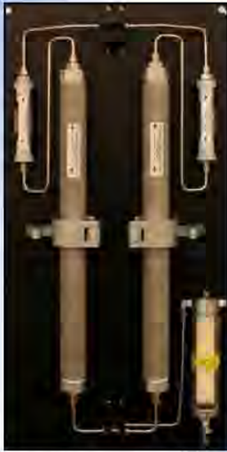
B-3251 H 2 S Scrubber System
