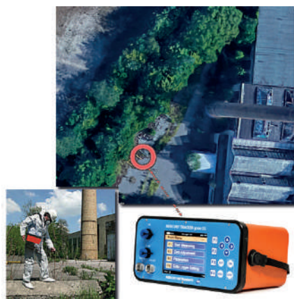
MERCURY LEAKAGE DETECTION
